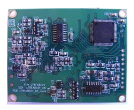
The uTRFABC23 is a RF coupler that fully comply to ISO 14443 Type A & B standard and ISO 18092 passive mode (or Sony Felica Type C) format. It can work with ISO 14443 type A, B and C compliance contactless smart cards.
