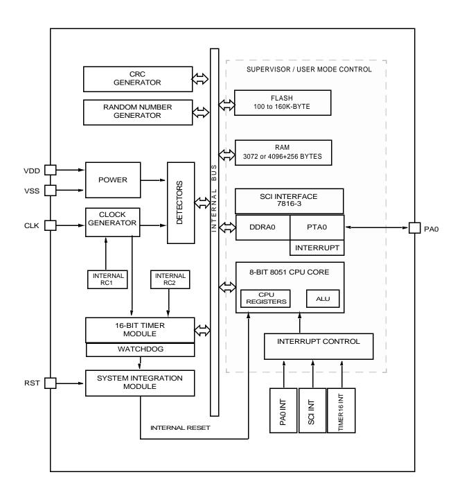
Figure 1. mT83SCA1XYS MCU Block Diagram
