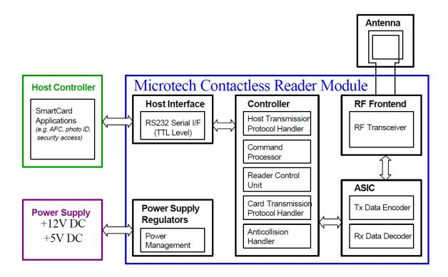
Figure 1: uTRFABC32 RF Coupler Block Diagram
